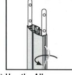
2) Use the Allen 3) wrench to attach the rails that connect the posts together
