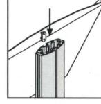
3) Slide the smaller rails (on 4) Tighten up the screws the back side of the literature in the literature t tray) down into the top of the trays lower pole's side channels
