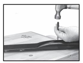
*Step 2a (optional).* Some of our posts fit very tightly together making it hard to turn the post to make the holes line up. If you received one like that, use the provided tool as a hole alignment tool by tapping it into the misaligned hole with a hammer.
