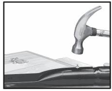
**Step 4:** Hit the drive rivet with a hammer until it looks like the image below.
