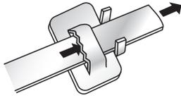
1. Pull appropriate length of band from BAND-IT Tote (approx. 3 1/2 times the diameter of the pole or mast arm for a single-wrapped clamp and double-wrapped clamp. Add 6 – 8 inches for both single-wrapped and double-wrapped clamps to accommodate the tail and bracket design.) Cut the band using one of the BAND-IT tools with built-in cutter. One end of the band will be very flat and the opposite end will be slightly bent from the cut-off.
