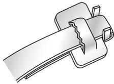
3. Squeeze the "lip wrap" to flatten the bend preventing "pull-out" during tensioning.
